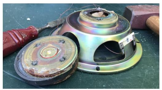
So with nothing to lose, I got to work with a hammer and chisel to separate the magnet assembly from the basket, a task I have done many a time in order to salvage the magnets.
