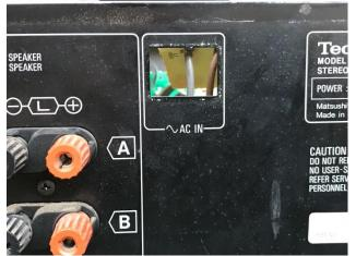
As you can see there is a bit of a void in the back panel – and a busted AC input sub-board inside.
