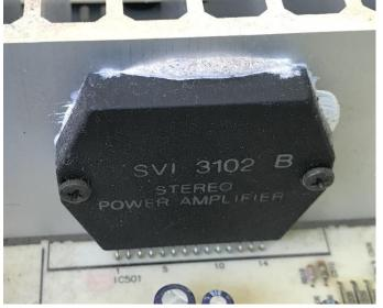
leaving the majority of the actual amp inside that plastic blob on the front of the heat sink – a heatsink with a bit more heft, aluminium wise, than is normally seen in medium power amps, with many using just sheet aluminium.
