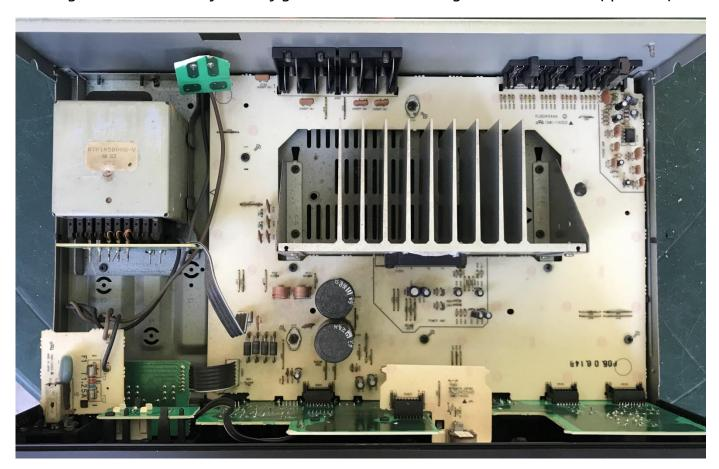
Inside, this has to be the emptiest/barest cases I've ever seen, where are all the parts? That little bit in the top corner is the phono pre-amp, the tone control circuits are on the front PCB,
