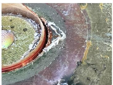
time it was so fouled that pulling off the magnet ripped the coil and its former right off the cone.
