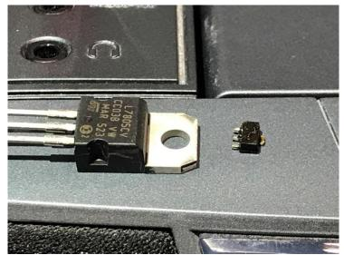
Once inside I soon realised it had tricked me, there was no switchmode supply, it was a boring old conventional iron core transformer based design, with a SMD 5V linear regulator to run the micro etc.
