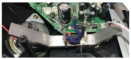
I fabricated a heatsink out of some aluminium flat bar I had.
