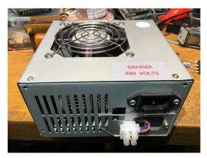
As it stands, with a fan (running as slow as possible) it was drawing 4.4W – Yikes, and with the load of 140mA that rose up to 12W, not good
