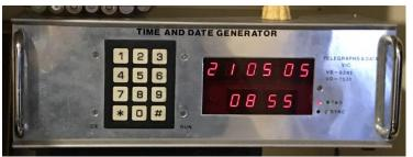
In my project to connect this old Baudo Time and date generator to the 'net (because everything is going to 'the cloud') I needed to convert its output to ASCII.
