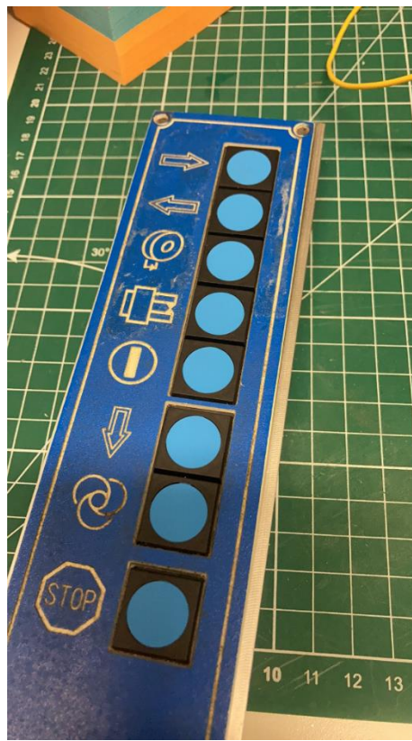
Pendant re-assembled with new PCB and existing faceplate and milled aluminium casing.
