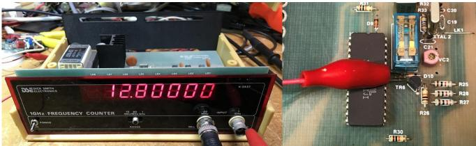
This will make the counter wrongfully display 12.8MHz, or rather it should, adjust the VC1 trimmer until it says 12.80000 and you're done. (The 1GHz input will not take a 10MHz signal)
