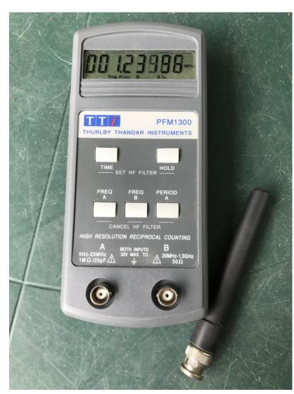
These days I use a portable frequency meter, a Thurlby Thander PFM1300, which goes from 5Hz to 1.3GHz, a somewhat better instrument than my old Dick Smith kit 1GHz counter. The latter has a horrible internal reference; it wanders all over the place, so is only good as a general check that you are not ridiculously off frequency.
