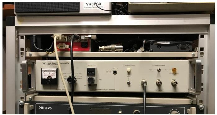
When working at the Telstra 'Equipment Services' repair shop, I was bitten by the frequency accuracy bug, and started collecting any relevant kit, which includes my last bit, a Trimble Thunderbolt GPSDO, or GPS Disciplined Oscillator, the red fronted bit of kit on the top shelf.
