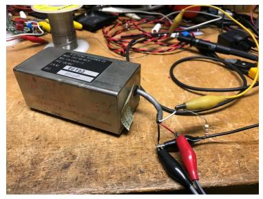
So what use is this if I don't have any of the flash gear that takes 10MHz I hear you say? Well there are more ways one can use this signal, the first is to calibrate the oscillators in your regular frequency counters, just shove it into the main input then adjust the trimmer in your counter so that it says 10.000000 MHz.
