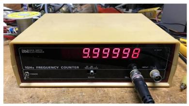
In the case of my Dick Smith K-3437 counter, I had to get sneaky, whilst the 10 & 80MHz range is easy to adjust, just feed in the 10MHz, the 1GHz range is not so. The 1GHz range uses a separate oscillator to allow for the odd division ratio of the 1GHz pre-scaler, 64:1.
