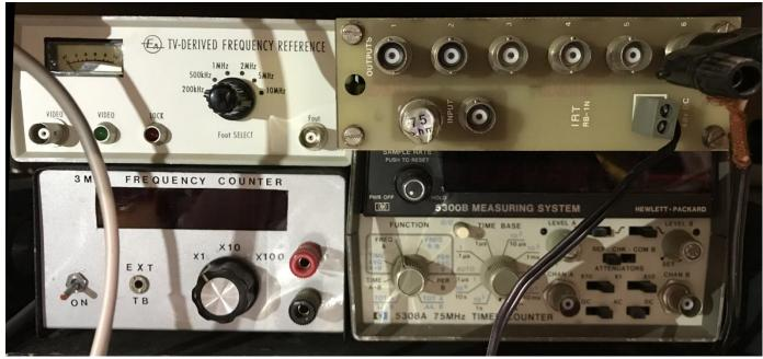
Second is a video distribution amp, they work great as 10MHz distributers. Next is probably the worst counter you could own, it uses the 50Hz mains as a reference – eek, EA what were you thinking. Last is a HP 5308A counter, pity it only goes to 75MHz, although it does accept 10MHz in on its back panel.
