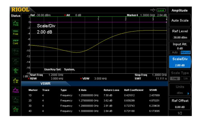
Next was to put some power into the dummy load, 120 watts @ 2M FM should be a nice test. After 5 minutes of continuous transmission the dummy load was only just warm. At 340 watts PEP on HF for 5 minutes the dummy load was the same. I'll have to clear some bench space before I go up a notch in power levels but it would appear at this stage that dummy load will be fine if kept within it's ratings.
