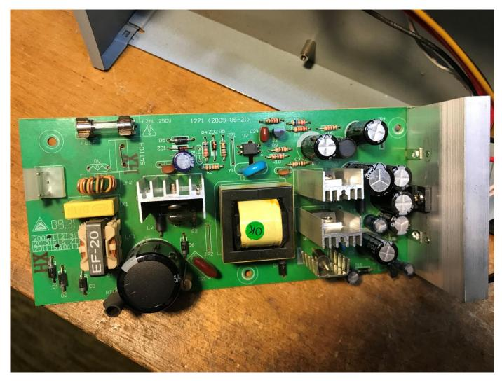
And here is the power supply, luckily easily extracted. The output cable to the main board had me a tad confused, it had two red wires, nothing unusual, a common trick done to lower the resistance & up the current, however my meter indicated that they were not connected to each other, unlike the two black wires.
