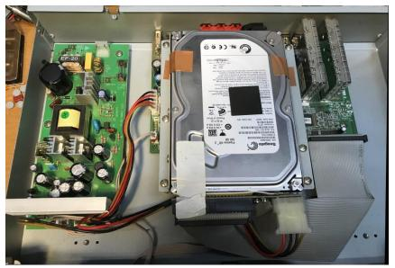
This PVR does have a standby button, however it does little, and does even less to the power supply that just pumps out 3.3, 5, & 12V as long as it is plugged in.
