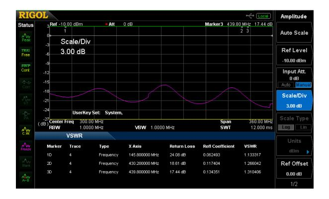
On the above sweep I tested 2M and 70cm, 2M came in with a VSWR of 1.13 to 1 and 70cm came in with a VSWR 1.31 to 1. Just for fun I swept the dummy load at 23cm to see what the results would be. As I expected, no good, after all the load is only rated up to 650 Mhz.
