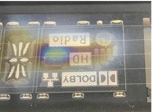
Closer inspection of the display however revealed that it was absolutely clapped out. You can see what looks like a metalized plating between the 'HD' and the first digit. That area is another square indicator, like the 'HD' one, that says 'TV'. It appears to be always on. The phosphor is all but gone, and what's left is masked by that plating. The adjoining digit does have top and bottom segments, again masked and totally hidden.
