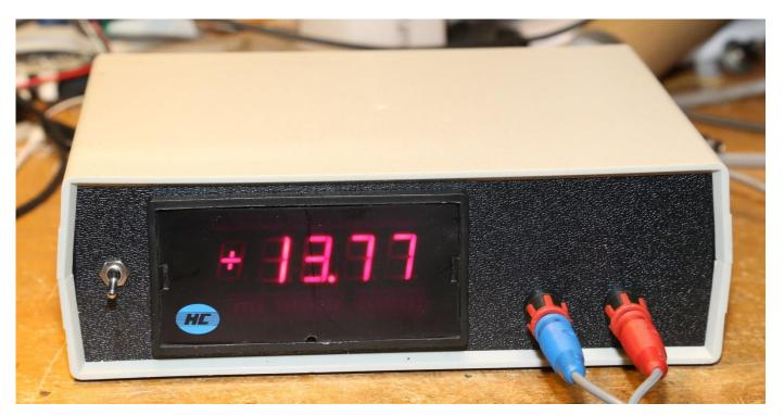
Another repair candidate. I was given this voltmeter, it's basically an industrial panel meter bunged into a standard plastic box. About the only thing the box is doing is to keep ones fingers away from the exposed terminal strip on the back of the meter module, exposed 240V terminals are a bit of an issue.
