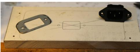
Here I am marking out the new back panel. The metal plate on the left is from someone else's hacks, but it sure comes in handy as a template for marking out. Some of the previous repairs, they just kept adding to the mess, rather than running a new wire directly into the fuse holder
