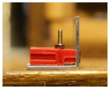
Here is how I generally chassis mount my Anderson power pole connecters. I cut a hole into some aluminium angle just large enough for the connectors to mate through; it is almost an interference fit. This way if there is any lateral pulling on the connecting lead, then the aluminium bracket supports the connector and takes most of that load.
