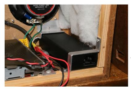
I looked through my junk box and ended up using a 7A switchmode power supply for 240V operation. I thought I had a 4A unit, a tad smaller, but that search ended badly.
