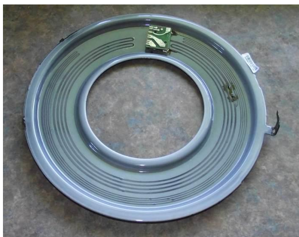
The heater pate with its vaporised section
