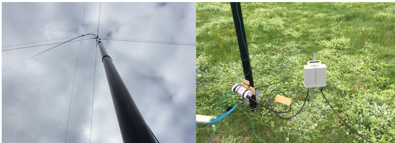
Figure 3 18m Spiderbeam mast, wire sloping to ground and match unit and LDG RT-600 tuner.
