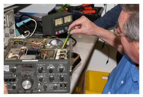
Now this is how it should be done, both to avoid detuning the radio by hanging that big chunk of metal off part of the PA output tank circuit, and to also avoid getting a lethal boot from the high voltages present in a valve output stage.
