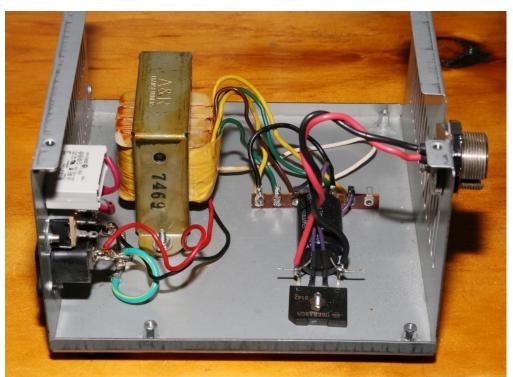
Speaking of the 180V supply, here is the temporary supply I built into an old computer power supply box.
