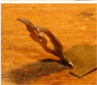
If the plug is not inserted squarely, then it can easily catch on the edge of the brass contact. All the user feels is a bit of resistance, so they push a bit more, and end up bending the contact and pushing it out of its housing.
