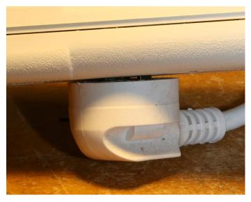
Here is a plug in one of those damaged sockets, apart from not feeling the plugs prongs make a double 'bump' as it passes the lower folded out sections, it is a tad proud of the face of the board. Now who runs their fingers around the base of the plug, or carefully looks across the board to make sure it's in all the way – Almost no one, except me, as I have grown accustomed to this cheaply produced junk. And what are your options, usually not much, as so many are built the same way.
