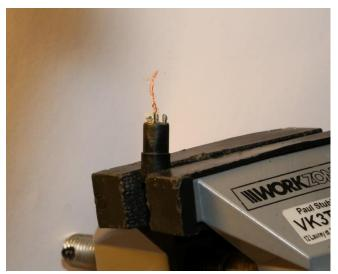
As I went I was using my multimeter trying to get continuity between the outer shield and what looked like the earth pin, Pin 3, on a mini Cannon plug. I kept getting closer, but could not see the break in the shield. I eventually got 99% of the resin/glue etc. off to reveal a wire soldered, a tad roughly, but soldered anyway to the plug solder bucket.
