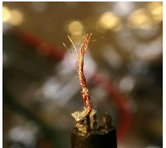
After much stuffing about it turns out that these are not thin strands of copper wire at all, Yes they are copper, but they are all individually coated with enamel, i.e. lacquered/enamelled winding wire, usually found in a transformer.
