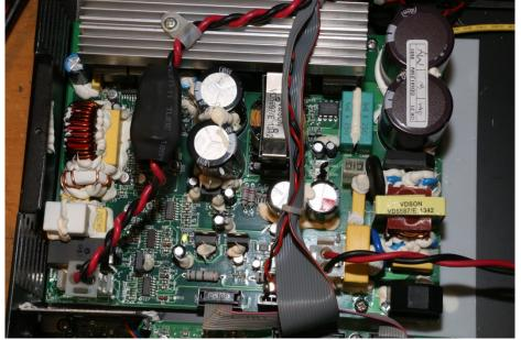
This is the main board, both power supply & audio amplifier on one board, it's actually quite scary to work on.
