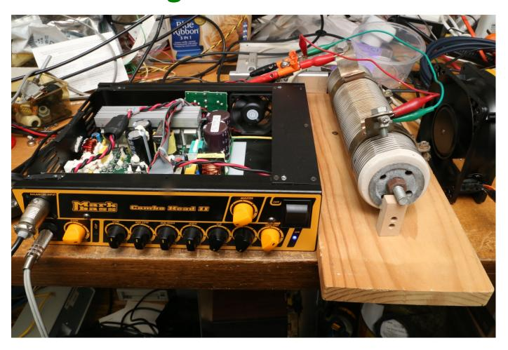
Recently I was given a "Mark Bass" bass guitar speaker/amplifier to repair. A quick check with a microphone (I am not a muscician – see I can't even spell it) Lots of distortion ensued, and the speaker cones seemed to be pulling inwards, so I kind of suspected a faulty output stage where either one of the output devices had failed, or we were missing a supply rail
