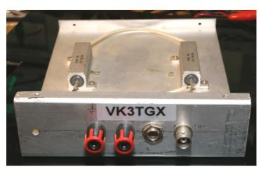
Normally to test an amplifier, I'll use a 6 ohm dummy load. I made up this one from some Telstra scrap years ago; however it was not going to cut it on this amp. I did run it for a short time but it got too hot far too quickly.
