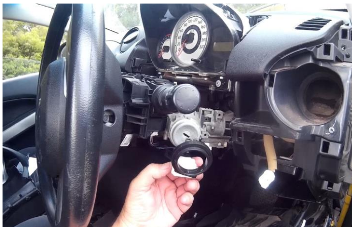
Removing the RFID Reader module & coil
