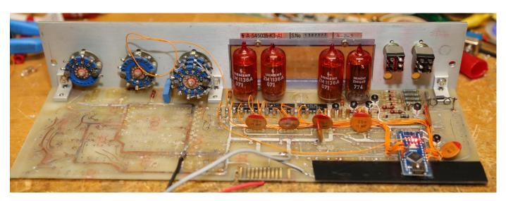
This is my recycled Siemens AK-001 Pulse measuring set (Hamfest special?) The black electrical tape under the Arduino Nano is to cover the HV line that runs from the edge connector right around the side of the board – no covering, just where I accidentally placed my finger YIKES!
