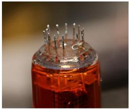
One surprise I had, was when I swapped the left hand tube from a 'symbol' tube to a regular 0-9 nixie, was that one of the wire leads had been accidentally crimped / folded over when it was inserted at the factory, and had been hiding there all along, never causing an issue.
