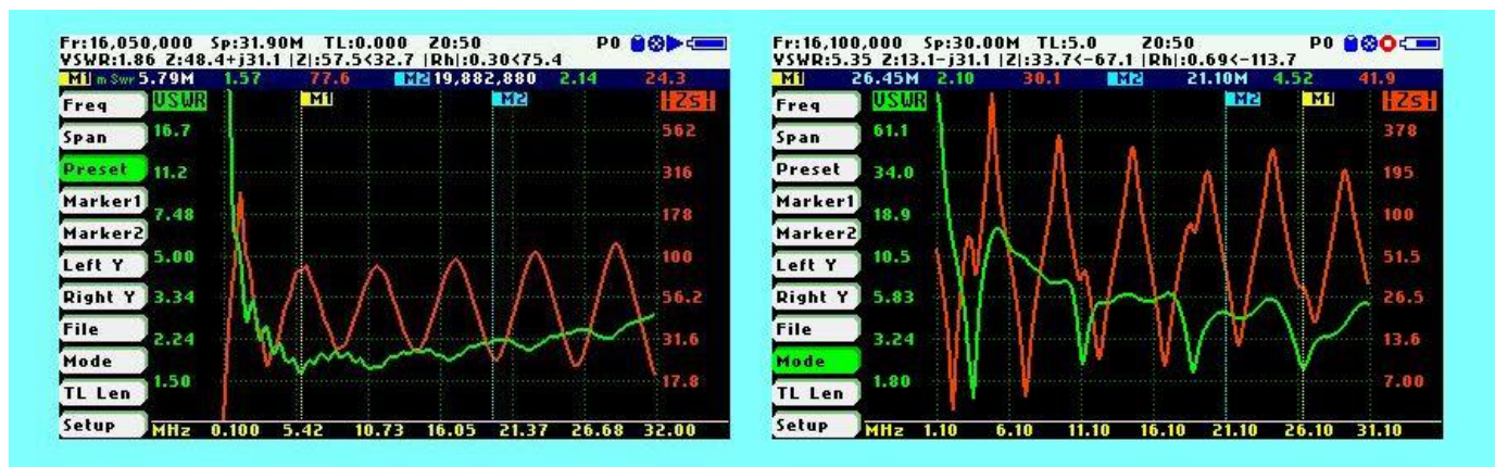
Left – the flat HF response of the Rhombic.
