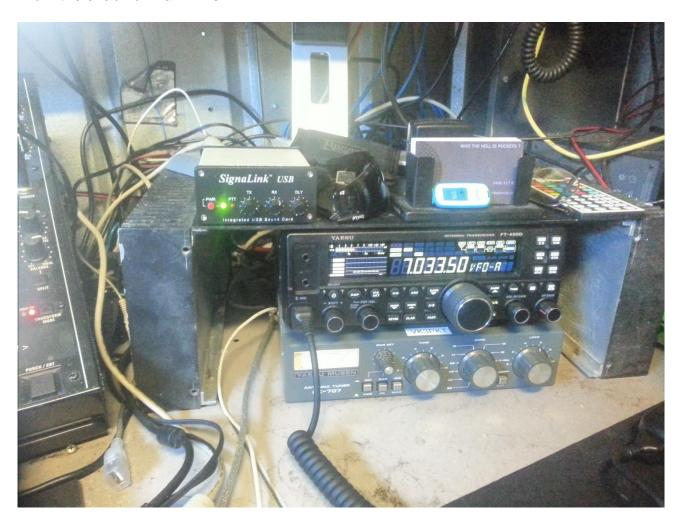
So just about 6 weeks ago I bought my first ever brand new HF rig for the twisted shack, it is a nice and shiny Yaesu FT-450D which is the latest model and comes with the built in ATU and digital filtering as standard.
