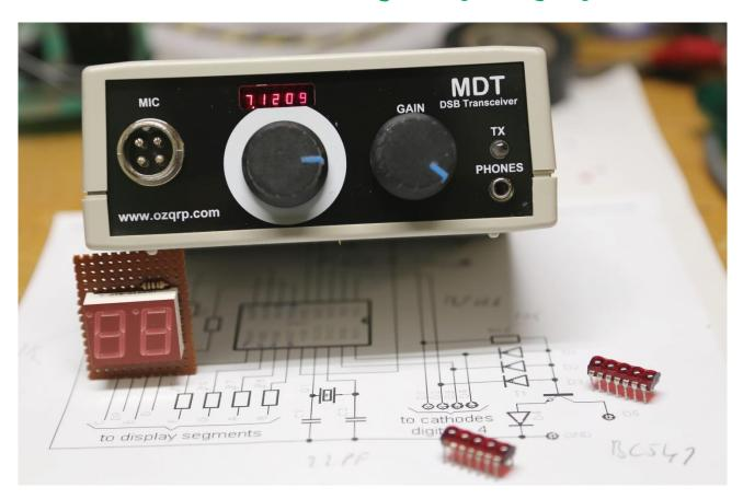
So you built the MDT radio kit, It's a nice little radio, however a frequency display it has not. I played around with mine at the anten... (hang on, copy,paste) Antennapalooza weekend at Ian's and I made some contacts, including one on Ian's Rhombic antenna, to a contest station, however I didn't have a pen and paper handy for a log – Hang on, what's one of the first things for the log – Frequency – oops, I haven't calibrated the dial.
