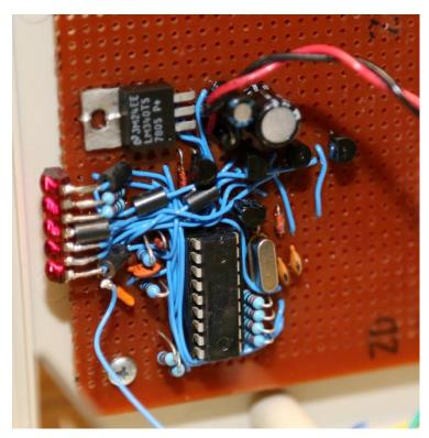
As you can see, I built mine on a piece of Varoboard with the display on the front edge so it shows through a window I cut just above the tuning control.
