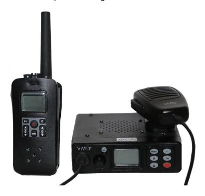
Later when using the Vivid radio, I found a big limitation. it loved picking up 70cm Amateur stations. As soon as I removed the lid all was revealed, it was almost empty; it would appear that they have simply put the innards of a very small hand held into a big box, alongside a 5W PA. The radio has no image rejection filters.
