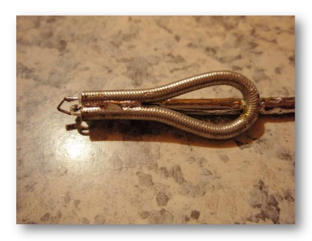
On the left hand end of the balun you can see 2 x 100 ohm SMD resistors (side on in a "vee" shape) in series that were used to tune the balun to 50 ohms feedline impedance. FYI the "hairpin" when straightened out is 85mm long (45mm for 13cm). Below shows the final sweep of the 23cm feedline and balun.
