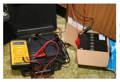
Later on, when the main battery hit 11.8V, I connected a second battery, this brought the DC volts back to up to a more respectable 12.15V
