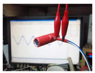
2 microphones will be used with the kit, one being the "speech" microphone and the other being the "noise" microphone. Adjustable Bass and Treble controls are included with additional adjustments being output level to the radio, degree of noise cancelling and the last being an adjustment to "balance" the noise cancelling circuit.
