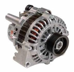
Falcon's, Hiluxes, Prado's and Klugers. These charge batteries to 14V when the engine is cold, but folds the output to around 13.4V when the engine has warmed up.
