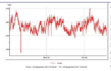
The image (left) shows a segment of a recording session taken at Philip Island last year where the mains bounced between 250 and 270V. The data logger tells a vivid story. Note the brief dip to 240 volts. This site had a generator which ran for 20 minutes on Sunday mornings as a test. At least it was generating the right voltage.
