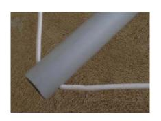
In the ends of the conduit a 4mm diameter hole was inserted to take the 2.5 sq mm insulated building wire. (in practise any old bit of wire will do) A good aspect of this design is that all the structural hardware is non-metallic and will not affect the optimal radiation pattern of the completed antenna.
