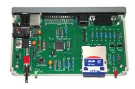
easy option of up to a 32Gig flash drive for storage then one of these may fit the bill. One way of looking at it is an intermediate step before going to a full PC (or laptop) The Maximite solves one problem of using a PC, size & power consumption. At 125mA you could run one on AA batteries, try that with a PC.
