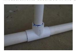
The boom is made from 60mm (outside diameter) PVC pipe. This is quite rigid and fits nicely into a standard 60mm Tee joiner.
